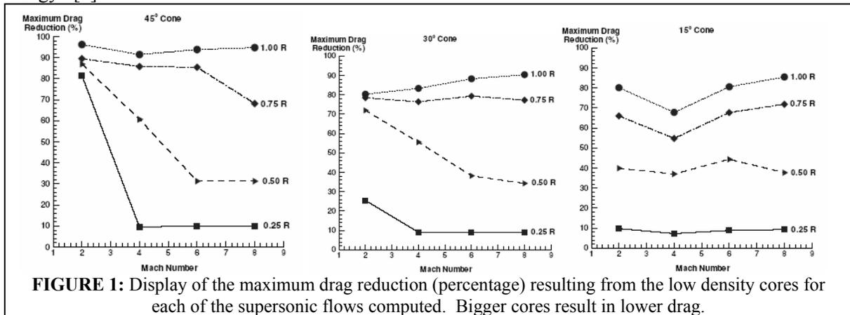
**FIGURE 1:** Display of the maximum drag reduction (percentage) resulting from the low density cores for each of the supersonic flows computed. Bigger cores result in lower drag.
