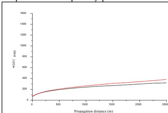
**FIGURE 6:** Simulation of a UV filament envelope diameter as a function of propagated distance, for an initial power of 160 MW. The filament diameter remains confined roughly within 100 microns over thousands of meters.[9]
