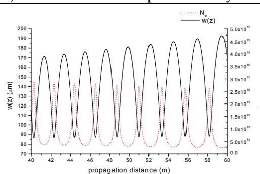
**FIGURE 5:** Simulation results of filament diameter and electron concentration as a function of propagated distance, for an initial power of 49.5 MW. Significant photoionization is seen only to occur over short lengths for which the beam confinement is maximum.[9]
