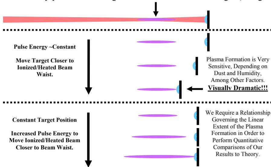
**FIGURE 12:** Two sets of measurements were performed to identify the effect of the heated core "connecting with" the shockwave from the laser-ablation. Top - using a roughly constant core length (roughly constant pulse energy), the target was moved toward the core. Bottom - keeping the target position constant, the core size was changed by varying the pulse energies.
