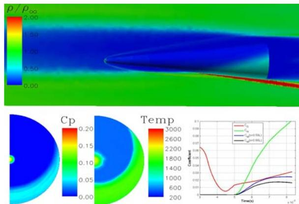
**FIGURE 10:** A frame of a test run using a standard cone to investigate the effects on heating, drag, and control forces when creating a hot low-density core ahead of a hypersonic vehicle's shock wave.
