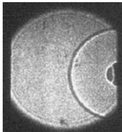
**FIGURE 11:** Shadowgraph image of shockwave from a nanosecond laser energy deposited in atmosphere on an Aluminum surface. Field of view, roughly 1.5"
